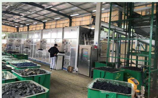
Low-temperature sludge drying and reduction equipment
